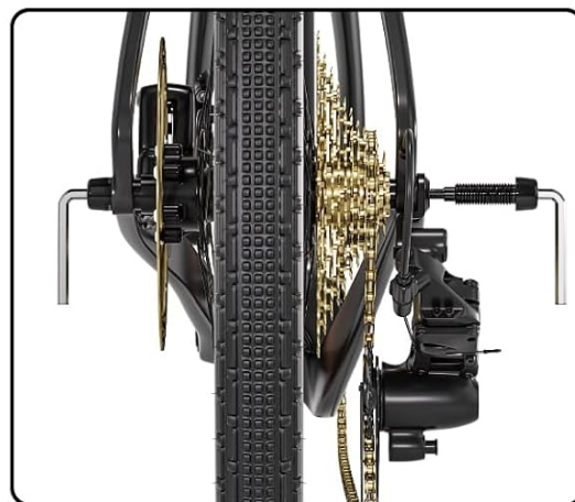
Image 4.1: Quick Release Skewer (A) and Thru-Axle Adapter (B) options for bicycle compatibility.
