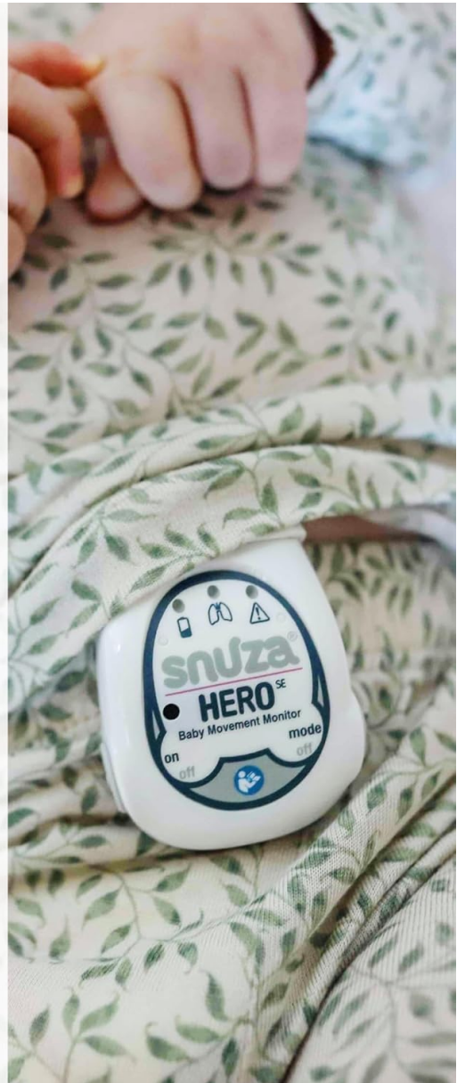
Image: Snuza Hero SE monitor attached to a baby's diaper, demonstrating proper placement.
