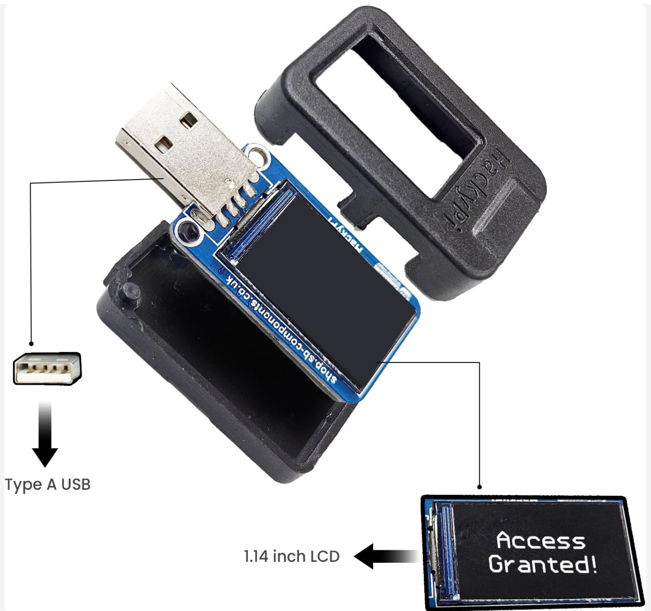
Image Description: An exploded diagram illustrating the internal components of the HackyPi, including the Type A USB connector, 1.14-inch LCD, 'Initiate Program' button, RP2040 MCU, and SD Card Slot.
