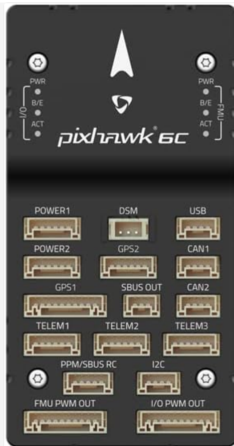
Image: Top-down view of the Pixhawk 6C, clearly labeling all input/output ports such as POWER1, POWER2, GPS1, GPS2, TELEM1, TELEM2, TELEM3, USB, CAN1, CAN2, SBUS OUT, PPM/SBUS RC, I2C, FMU PWM OUT, and I/O PWM OUT.
