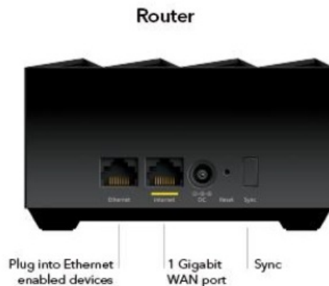
Image 3.1: Back panel of the Nighthawk Router, showing Ethernet ports for devices, a 1 Gigabit WAN port for internet connection, DC power input, Reset button, and Sync button.
