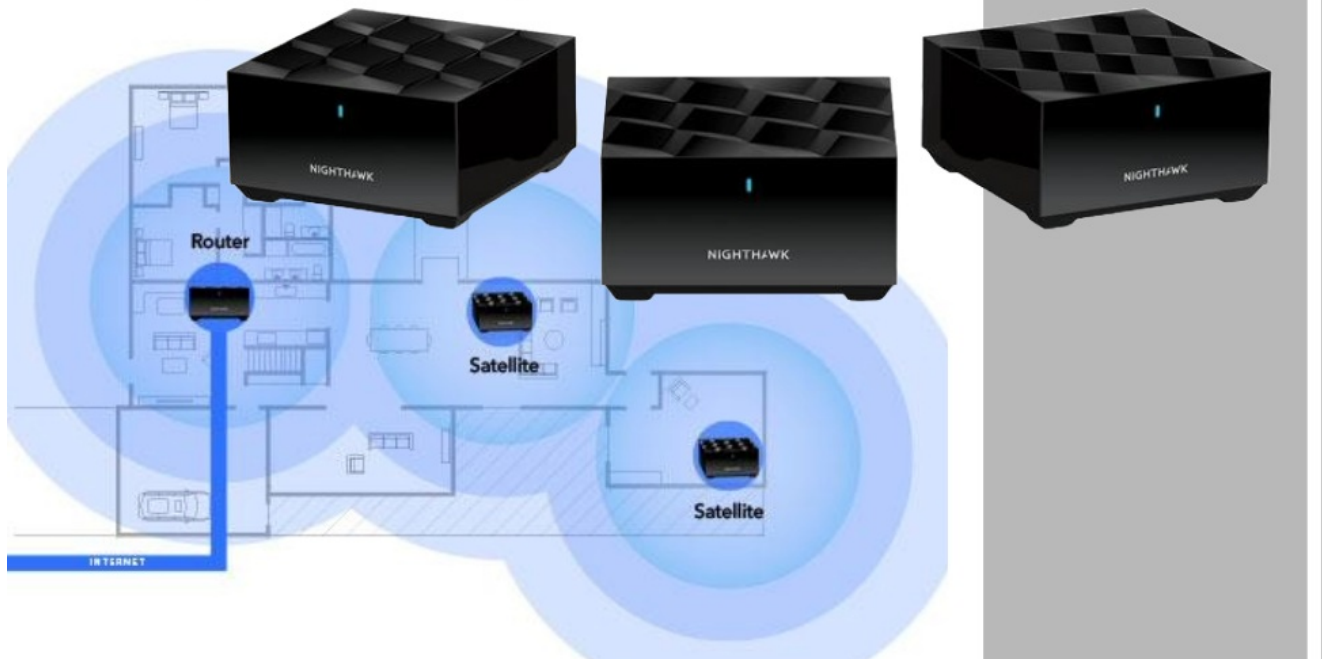
Image 4.1: Diagram illustrating the placement of the Nighthawk Router and Satellites to achieve advanced WiFi 6 coverage up to 4,500 sq. ft. throughout a home.
