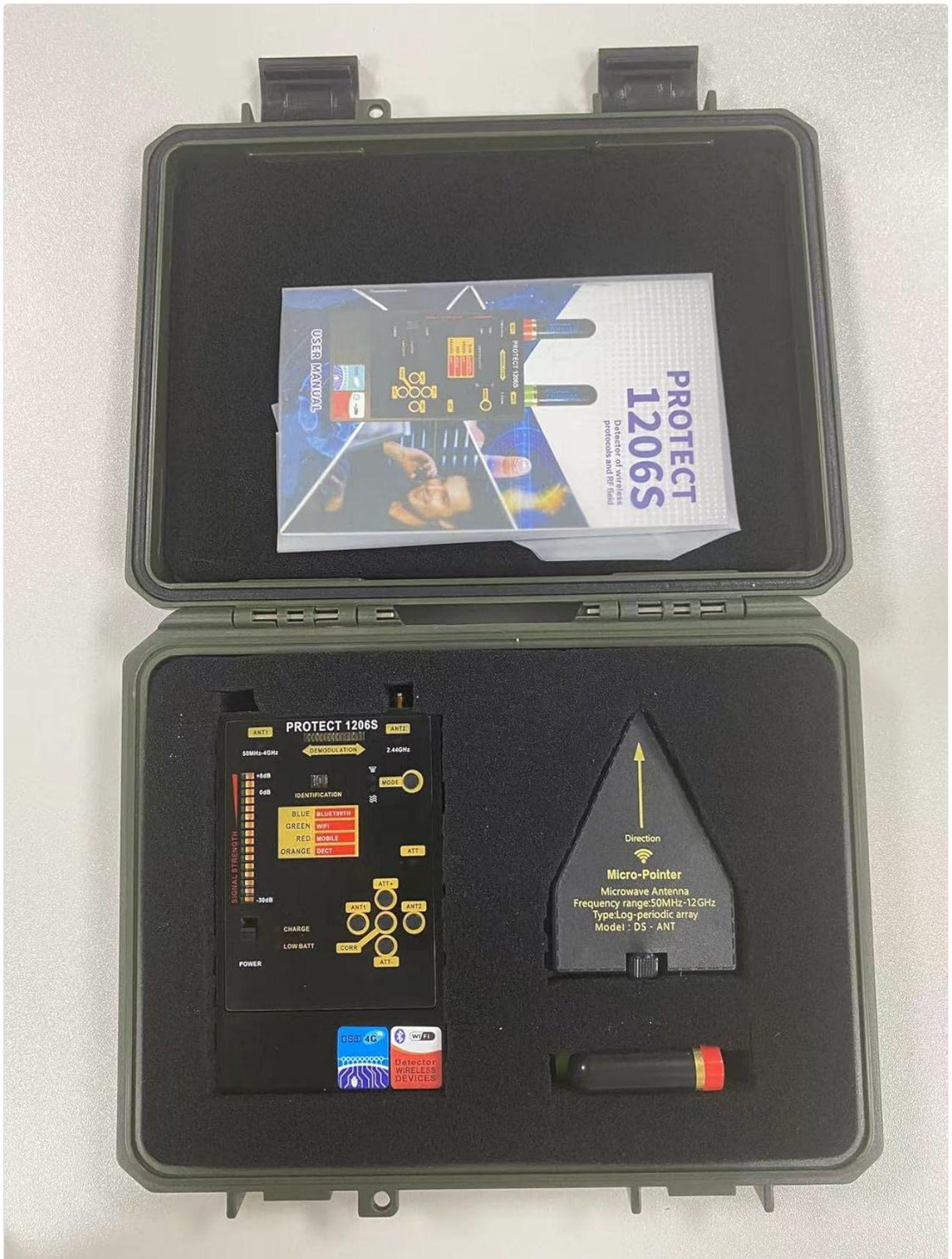
Figure 4: Protect 1206S in its Protective Case. This image shows the detector, antennas, Micro-Pointer, and user manual stored within a durable, olive-green protective case, highlighting its portability and secure storage.
