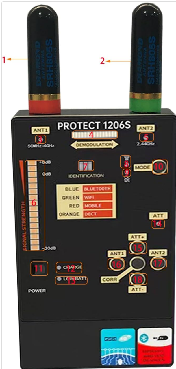
Figure 1: Protect 1206S Detector Components. This image displays the front panel of the Protect 1206S with numbered labels pointing to various indicators and controls, including antennas, signal strength meter, identification lights, mode button, and power switch.
