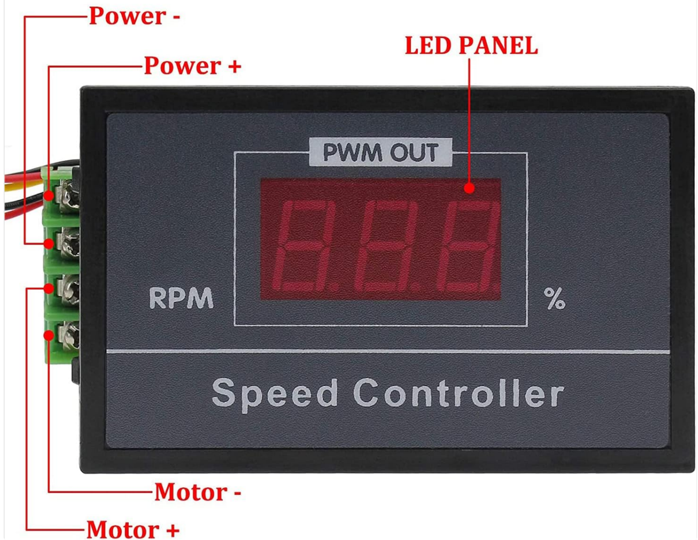
Figure 4: Wiring diagram for the speed controller.
