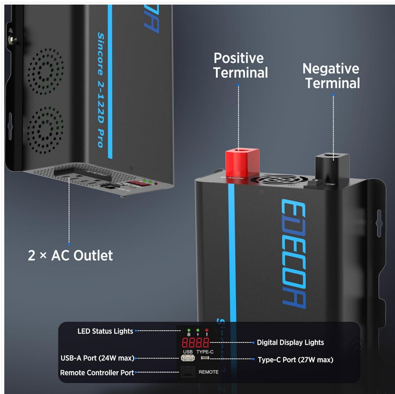
Detailed view of the inverter's front panel, indicating the location of AC outlets, USB and Type-C charging ports, LED status indicators, and the digital display.
