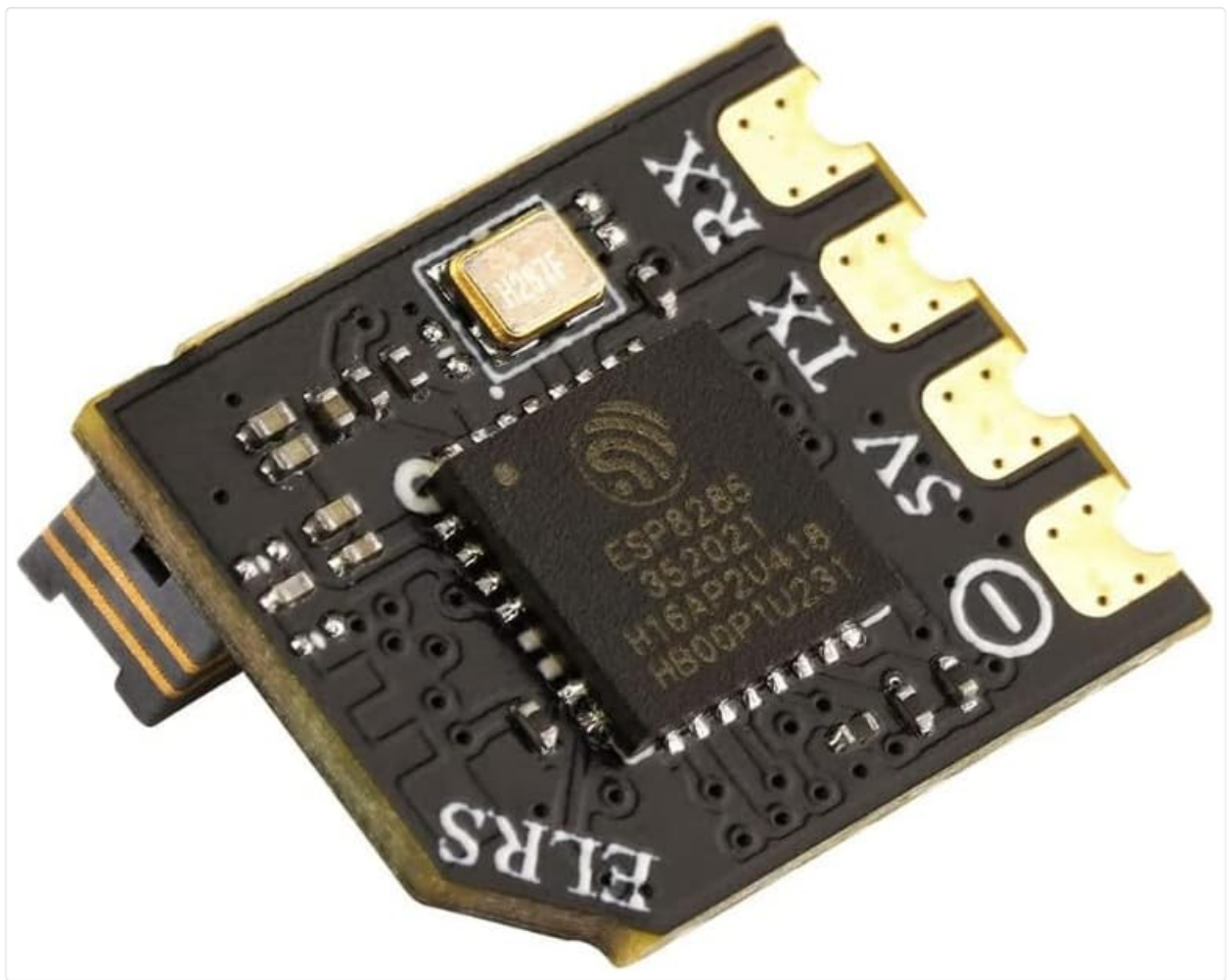
Image: Bottom-up angled view of the RP2 receiver, showing the ESP8285 chip and additional components on the underside.
