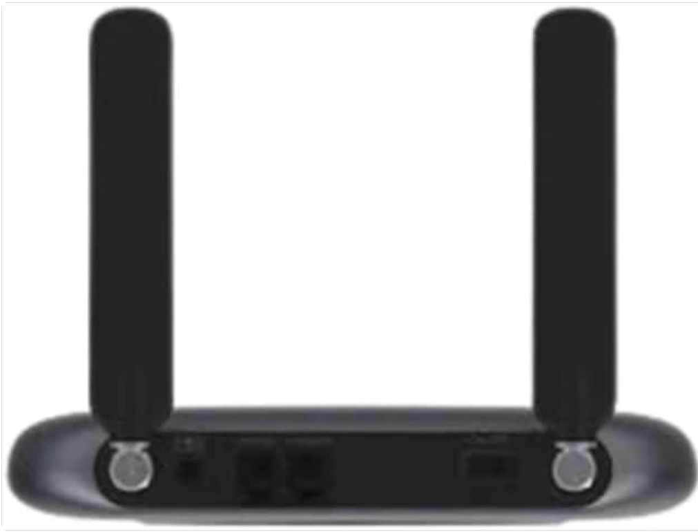
Image: Rear view of the ZTE WF723 Wireless Home Phone Base, displaying the two RJ11 phone ports, power input, and external antenna connectors.
