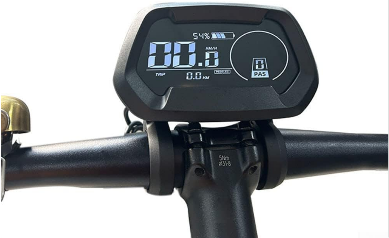
Image: The DZ43 display mounted on a handlebar, illustrating its position and the visible USB charging port for convenience.
