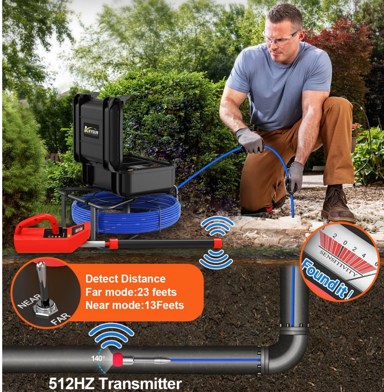
Figure 5: The 512Hz locator receiver being used to pinpoint the camera's location. The camera probe emits a 512Hz signal, allowing the receiver to accurately detect its position and depth.
