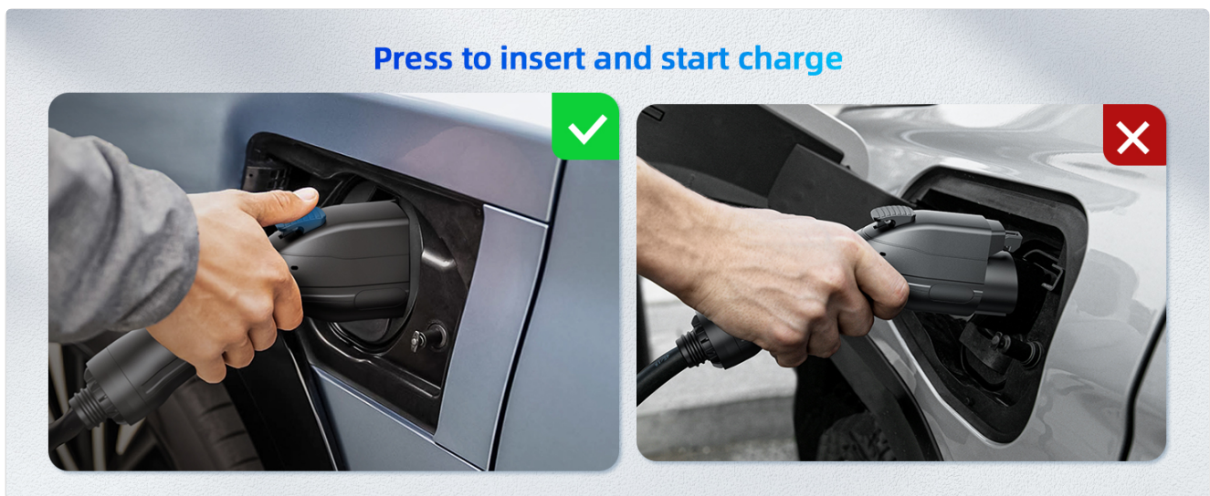
Figure 8: Correct method for inserting the charging connector.
