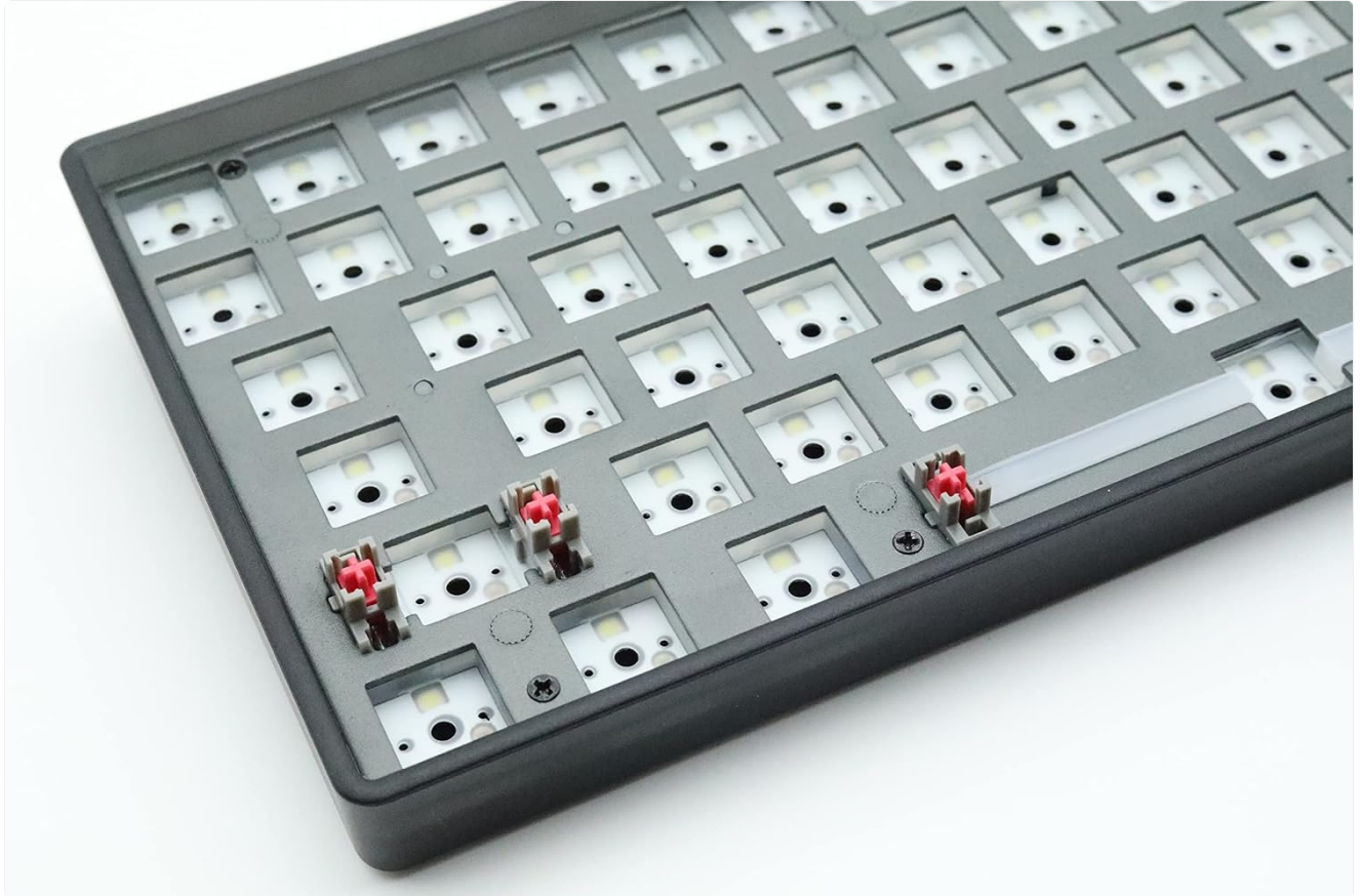
Image: Keyboard PCB with hot-swappable sockets ready for switch installation.
