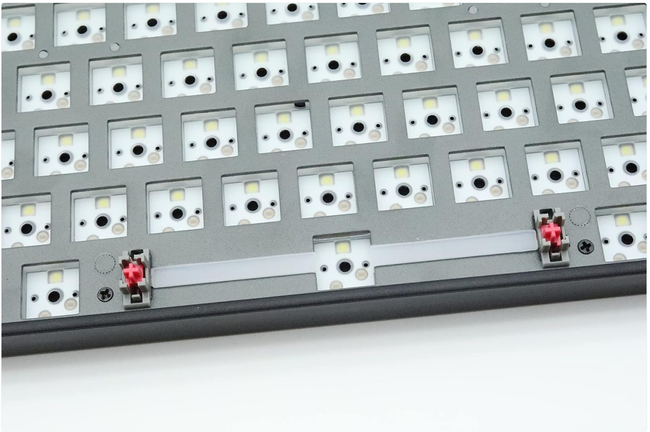
Image: Detailed view of a hot-swappable switch socket and stabilizer.
