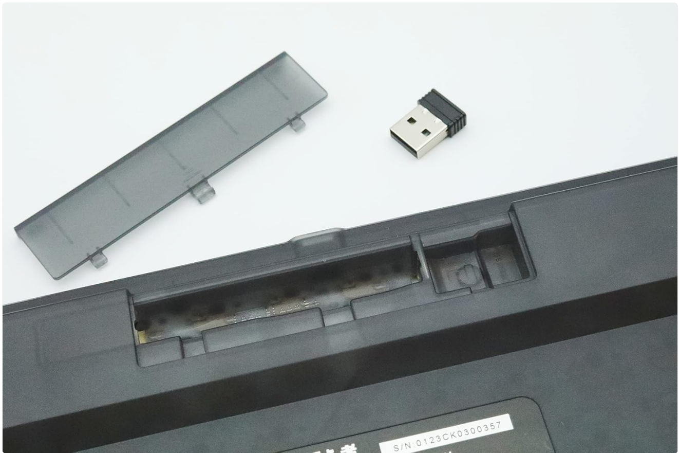
Image: Battery compartment and 2.4G USB dongle storage.
