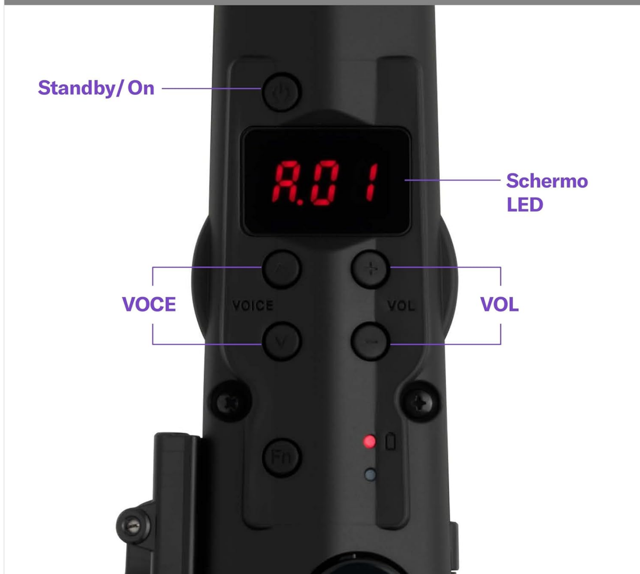
Figure 3.2: Detailed view of the YDS-120's control panel, showing the Standby/On button, LED screen, VOICE selection buttons, and VOL (volume) buttons.
