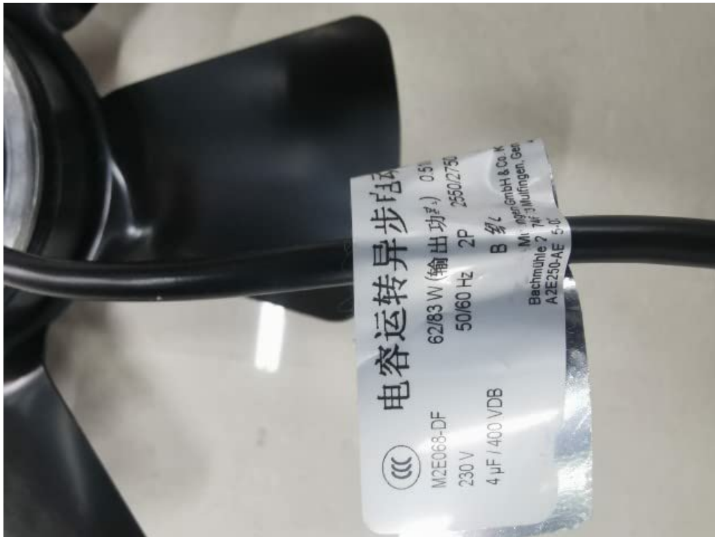
Figure 2: Close-up of the fan's wiring and specification label.
