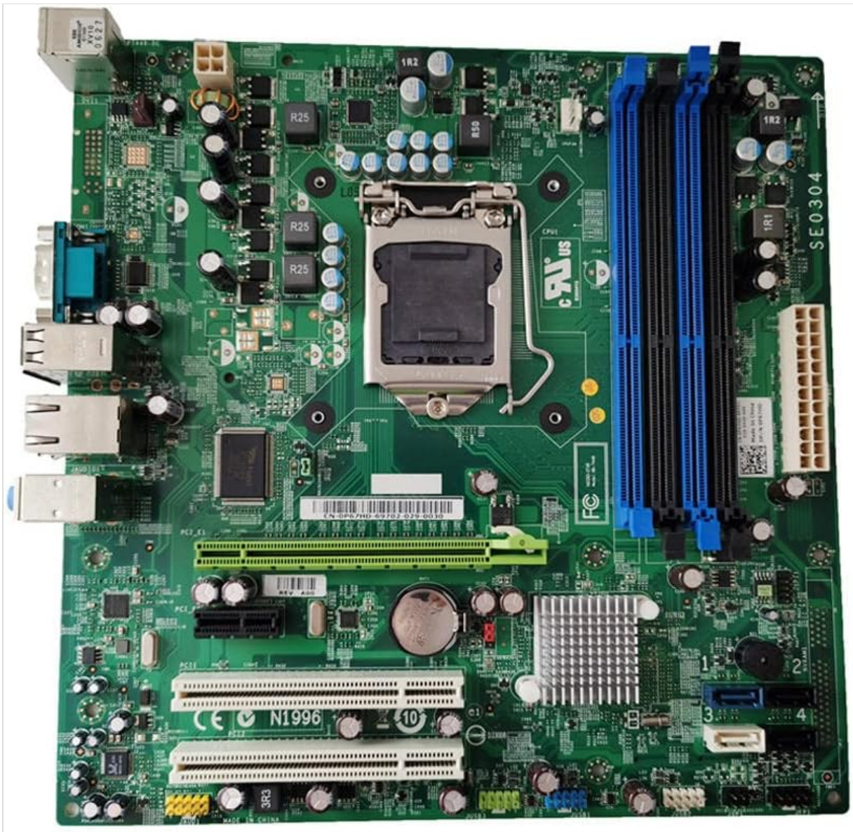
This image displays the overall layout of the motherboard, including the CPU socket, memory (RAM) slots, and various expansion slots.
