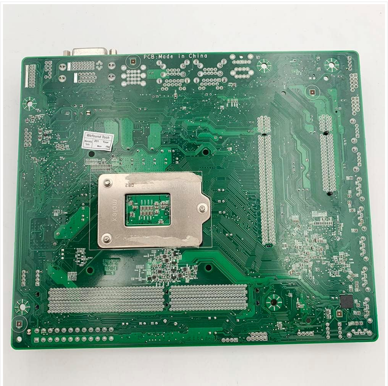
Figure 4.1: This image displays the back of the server motherboard, featuring the central CPU socket, multiple memory DIMM slots, and the intricate circuit board design. This view is crucial for identifying component placement during installation.
