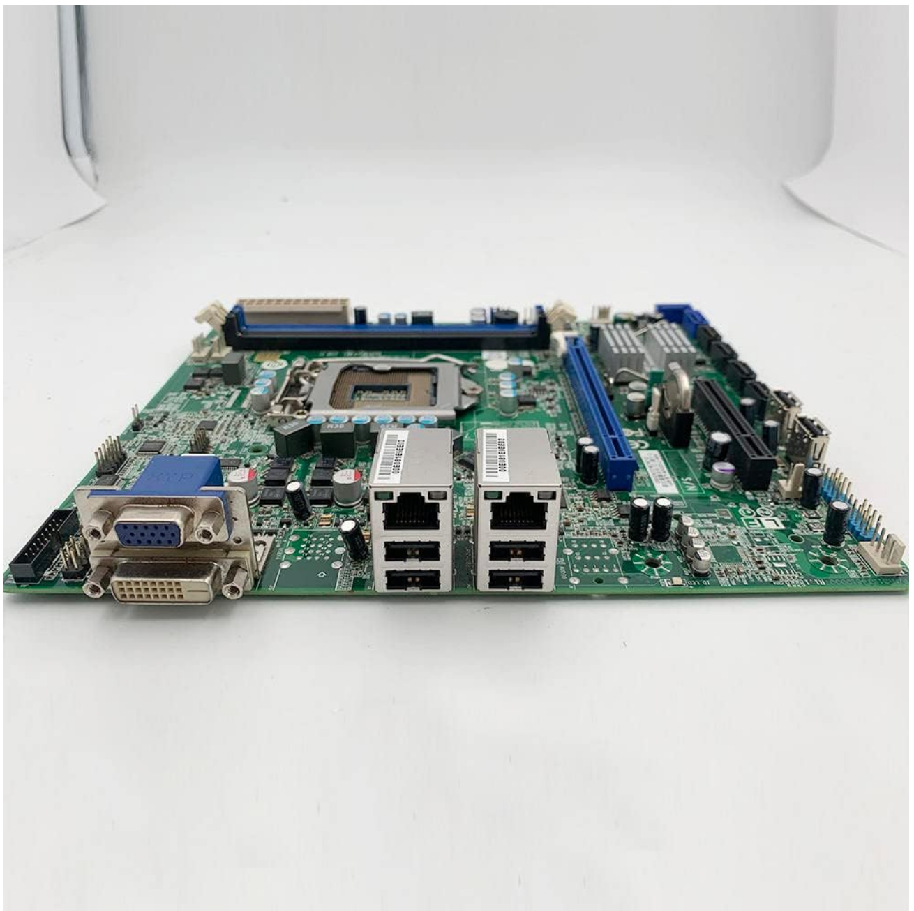
Figure 2.3: This side view illustrates the motherboard's input/output (I/O) panel, featuring VGA and DVI video outputs, dual Ethernet (LAN) ports, and USB ports. These ports are used for connecting peripherals and network cables.
