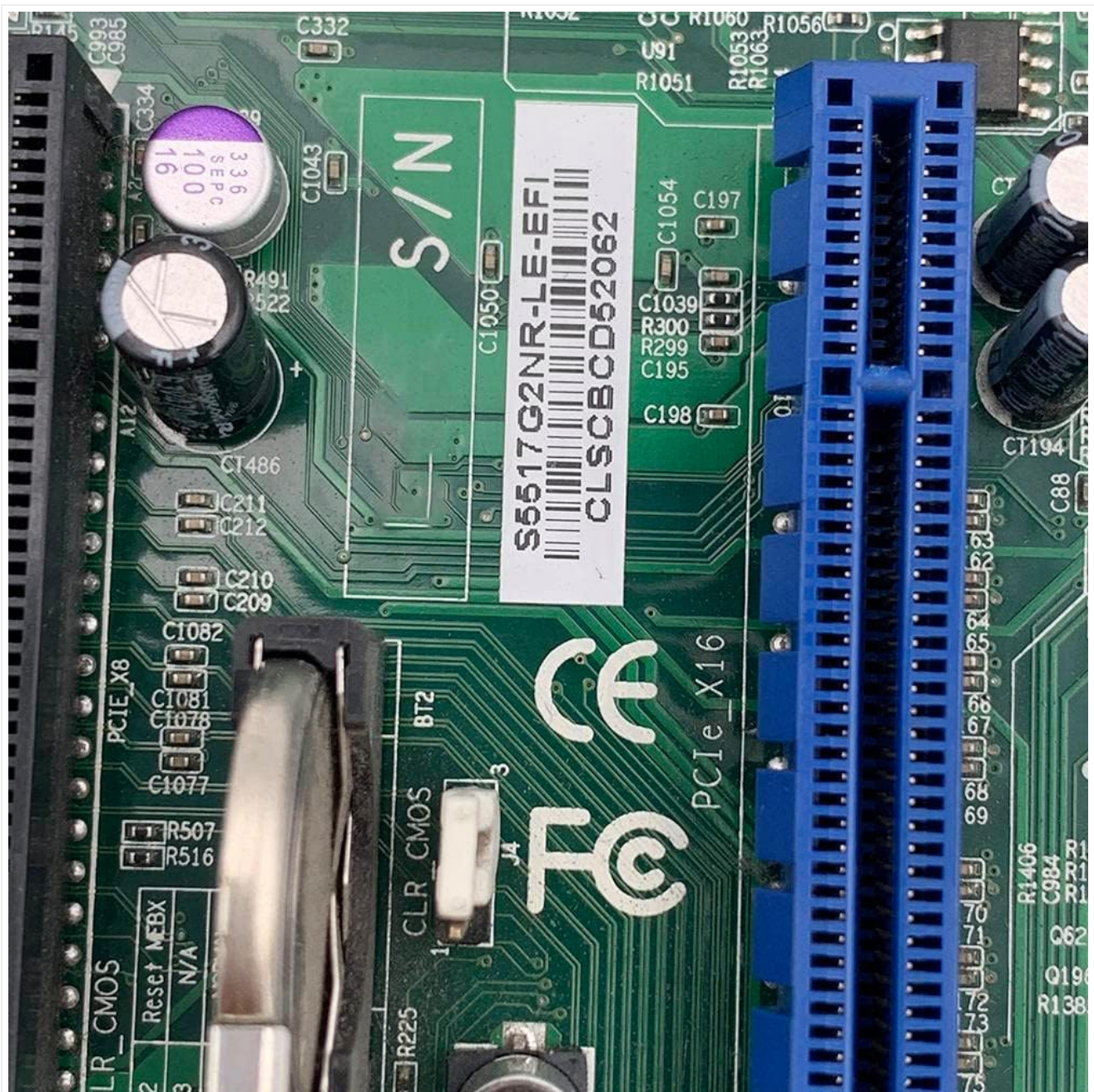
Figure 4.2: This image highlights the PCIe X16 and PCIe X8 expansion slots, along with a serial number barcode. These slots are used for installing expansion cards such as graphics cards or network adapters.
