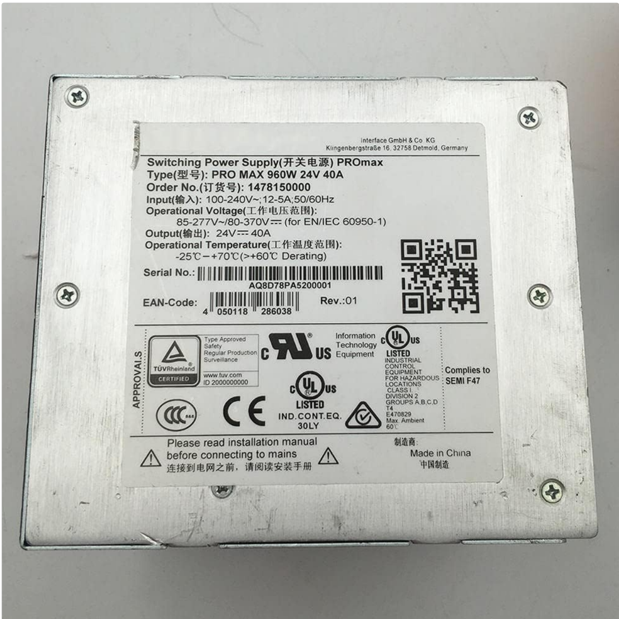
Figure 3.1: Product label detailing input/output specifications, operational voltage, temperature range, serial number, EAN code, and various safety certifications (TÜV Rheinland, UL, CE, CCC).
