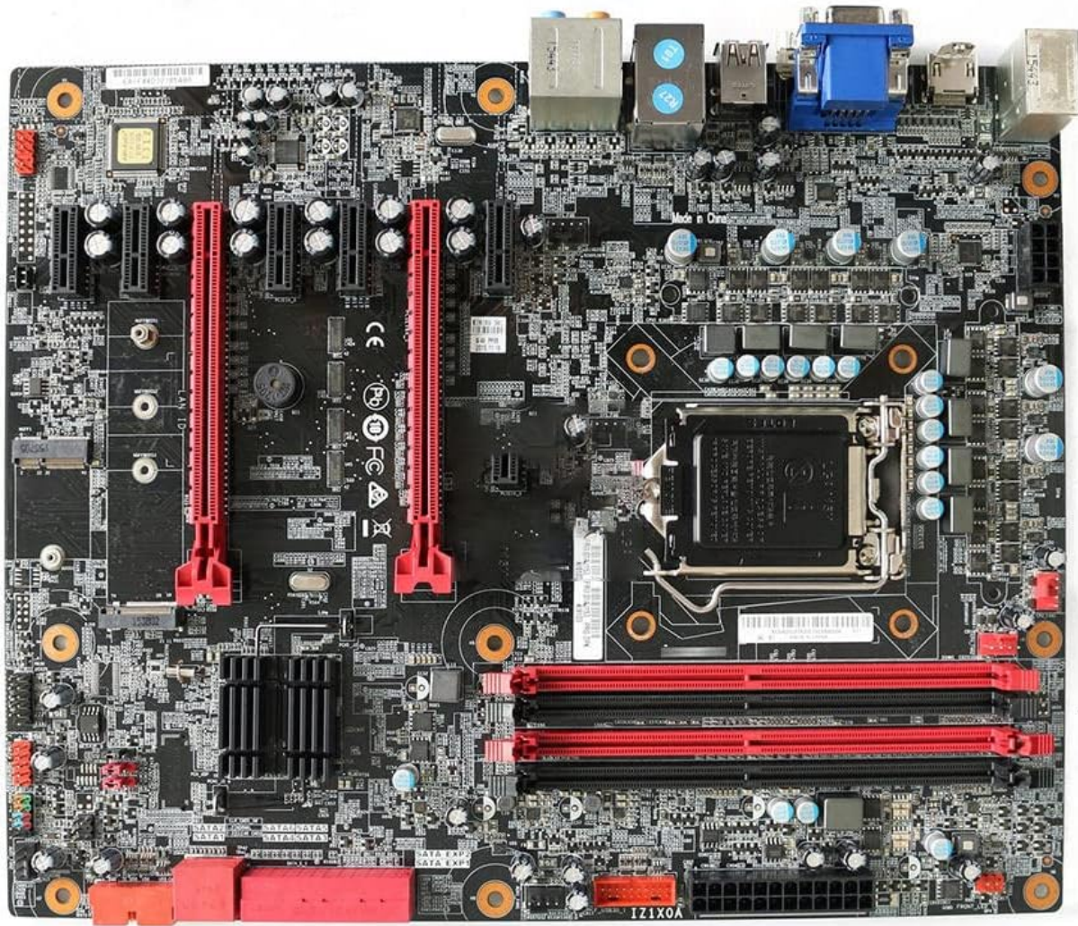
Figure 1: Front view of the Generic Z170 Y900-34ISZ Desktop Motherboard, showing CPU socket, RAM slots, PCIe slots, and various connectors.
