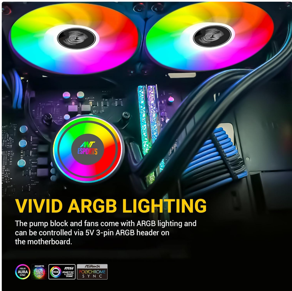
Image 7.2: The pump block and fans feature vivid ARGB lighting, controllable via motherboard software.
