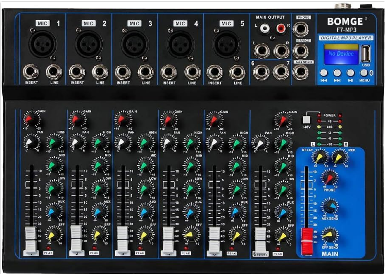
Figure 1.1: Front view of the BOMGE K7 7-channel Bluetooth Portable Audio Mixer, showcasing its various input channels, faders, and control knobs.
