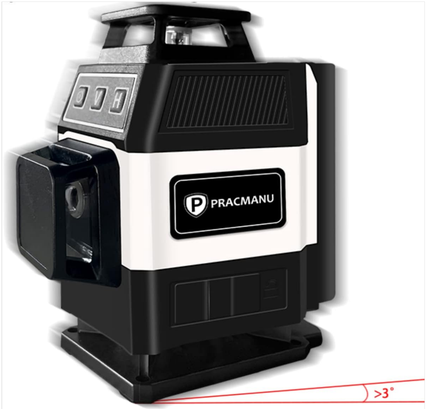
Figure 4: Illustration showing the laser level indicating an angle greater than 3 degrees, which causes the laser lines to flash, signaling that it is outside its self-leveling range.
