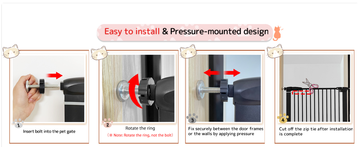
Figure 4: Installation Steps. 1. Insert bolt into the pet gate. 2. Rotate the ring (not the bolt) to adjust. 3. Fix securely between door frames or walls by applying pressure. 4. Cut off the zip tie after installation is complete.
