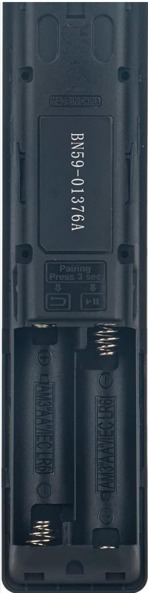
Image: Rear view of the remote control with the battery cover removed, illustrating the correct placement for two AAA
