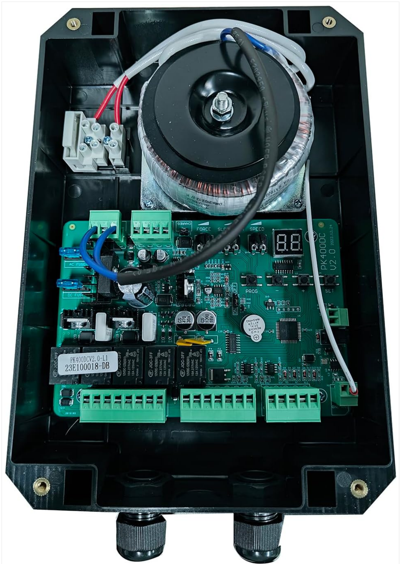
Figure 3.2: Gate Opener Motors and Control Box
