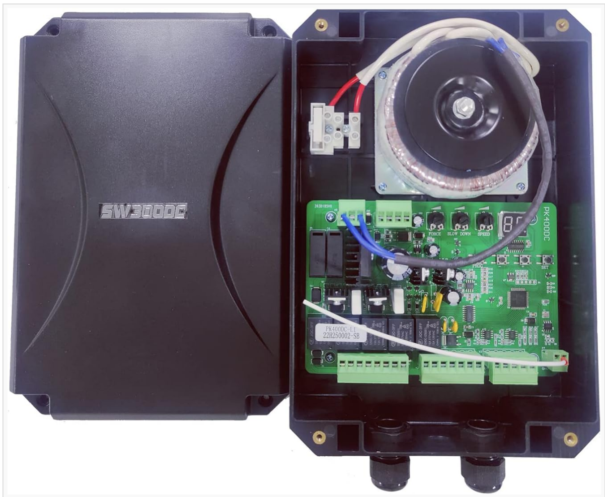
Figure 6.1: Internal view of the GATEXPERT SW300DC control box, showing the circuit board and transformer.
