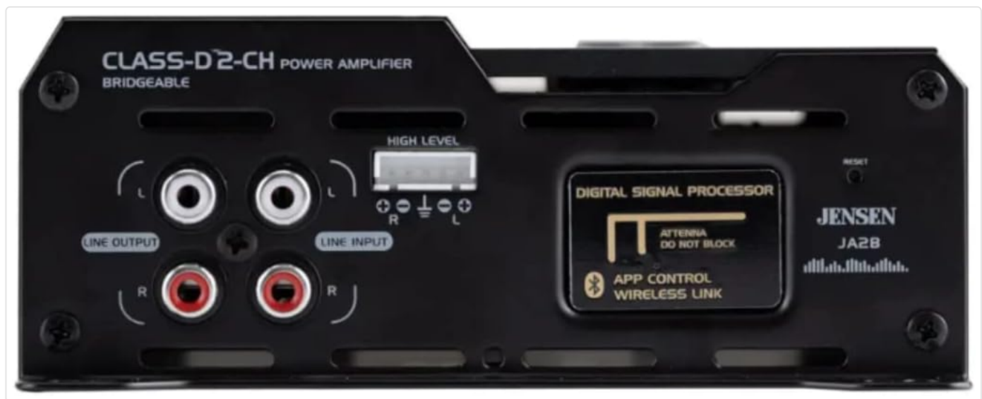
Figure 4: Rear panel of the Jensen JA2B amplifier, showing the High-Level input, Line Input (RCA), Line Output (RCA), and the Digital Signal Processor (DSP) section with app control wireless link indicator.
