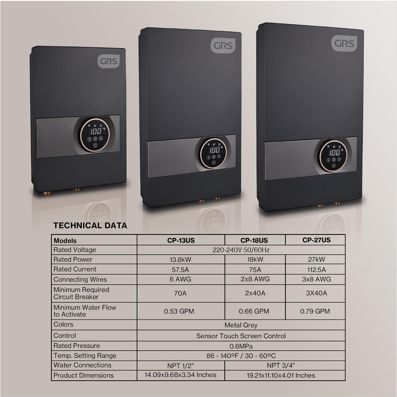
Figure 4: Technical Data for GRS Tankless Water Heater Models. This table provides detailed specifications for the CP-13US, CP-18US, and CP-27US models, including rated voltage, power, current, wire size, circuit breaker requirements, and dimensions.
