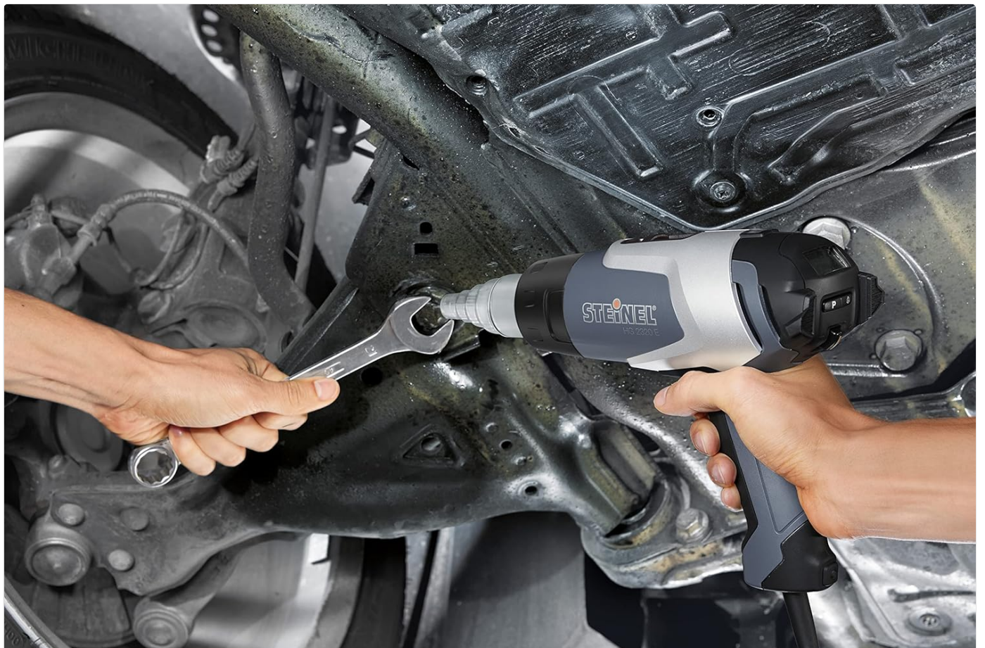
Image: The heat gun being used to loosen a stubborn bolt on a vehicle, showcasing its versatility.
