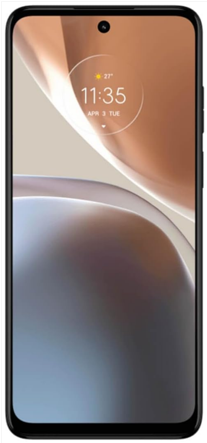
Figure 1: Front View. This image shows the front of the Motorola Moto G32, highlighting its 6.5-inch display and the front-facing camera cutout at the top center.
