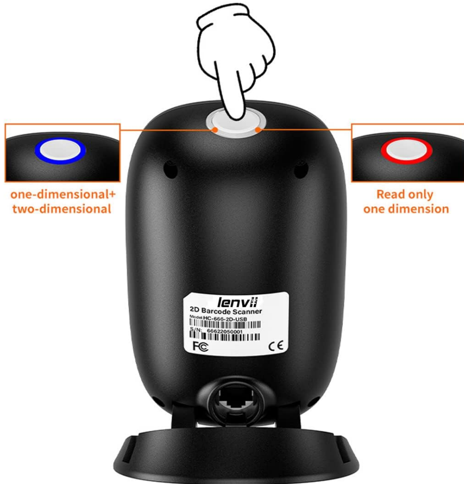
Figure 4.1: Instructions for switching reading modes on the LENVII D2200. Pressing the top button toggles between "one-dimensional + two-dimensional" (blue light) and "read only one dimension" (red light) modes.
