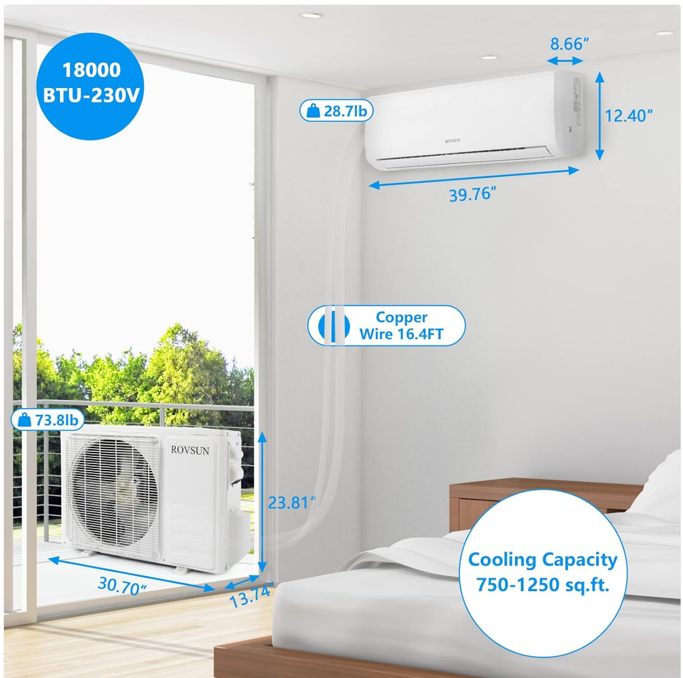
Figure 8.1: Dimensions and specifications for the 18,000 BTU-230V model.
