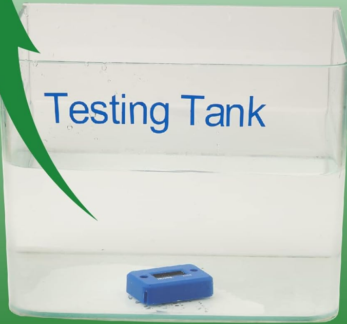
Image: The hour meter fully submerged in water during a waterproof test.
