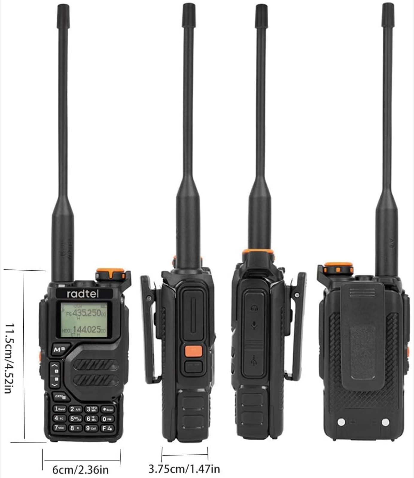
Figure 7.1.1: Dimensions of the Radtel RT-590 Walkie Talkie, showing height and width measurements.
