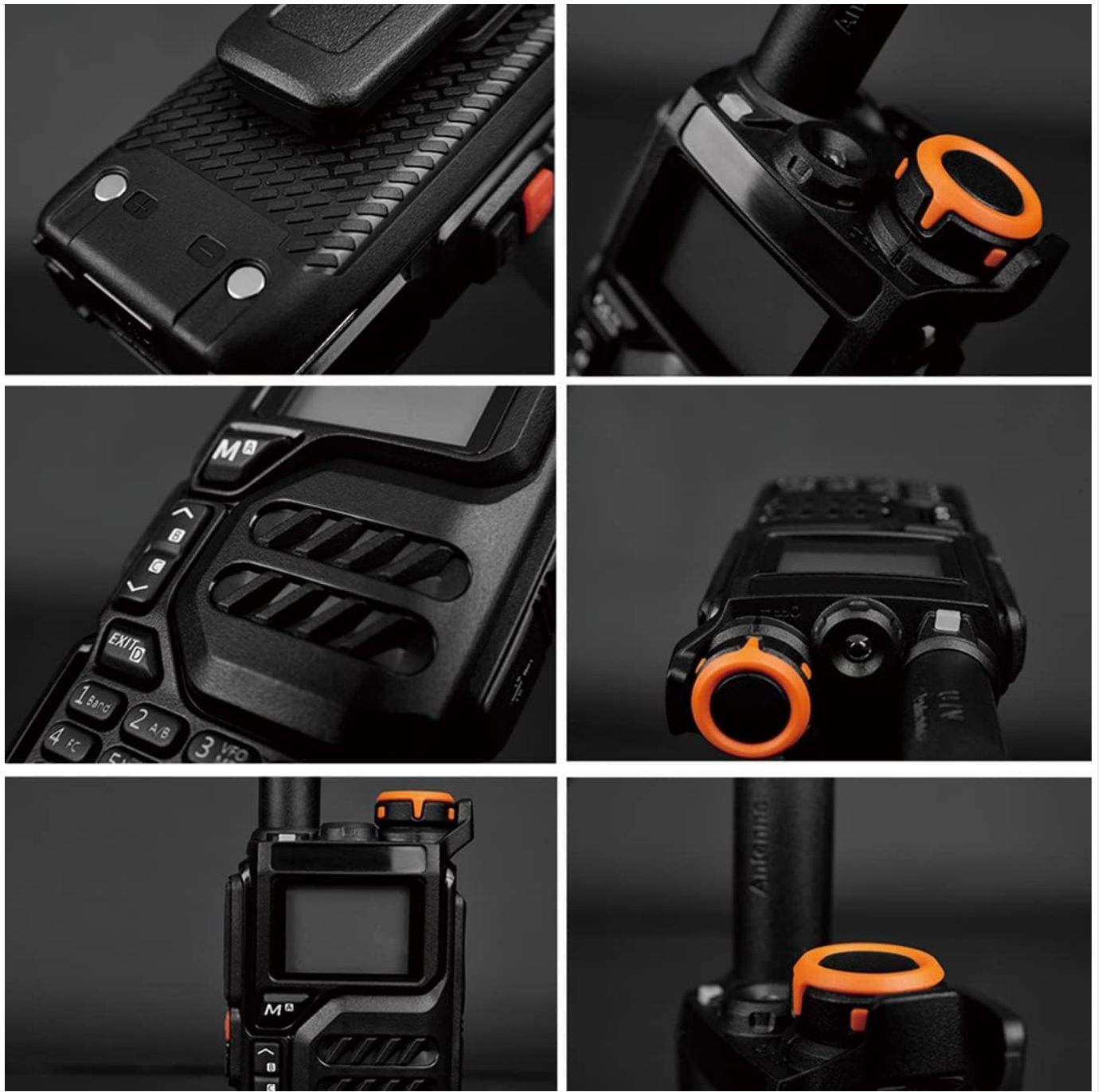
Figure 2.3.2: Detailed views highlighting various parts of the RT-590, including the belt clip, top knob, side buttons, and charging port.
