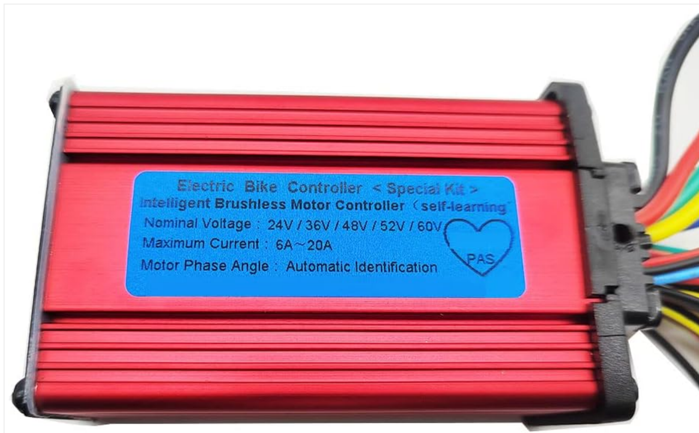
Image: Close-up of the label on the ChongXiao Electric Bike Controller, indicating it is an Intelligent Brushless Motor Controller with self-learning capability, nominal voltage range of 24V/36V/48V/52V/60V, maximum current of 6A~20A, and automatic identification of motor phase angle.
