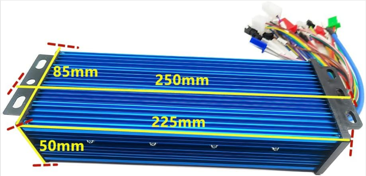
Figure 5.1: Controller with key dimensions.
