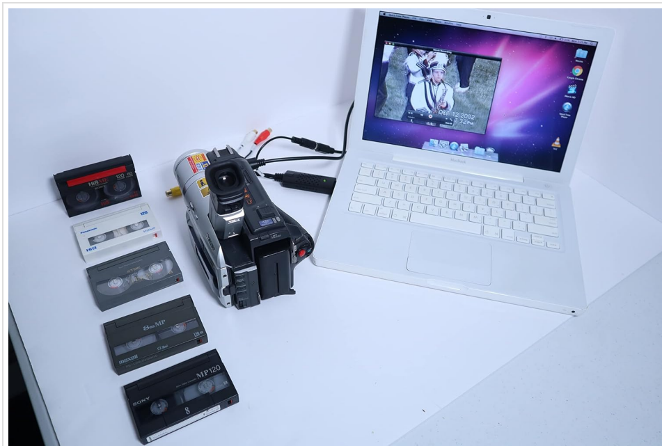
Figure 4: Camcorder connected to a laptop for video digitization.
