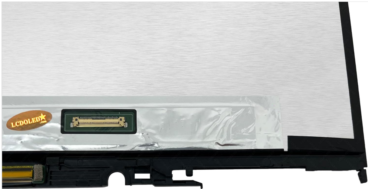
Figure 3: Detailed view of the EDP 30-pin connector and the integrated touch control board, crucial for display and touch functionality.
