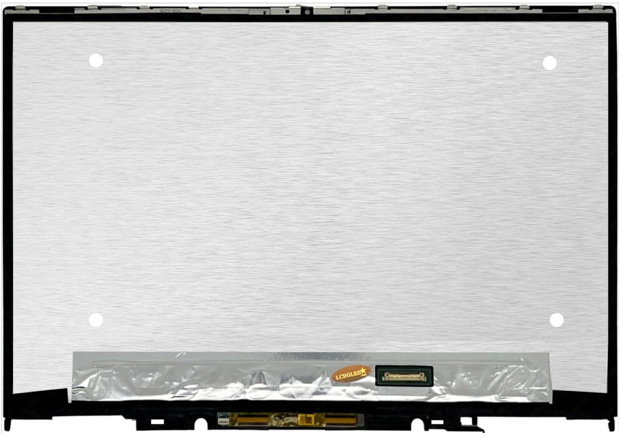
Figure 2: Back view of the LCD/LED replacement display assembly, highlighting the mounting points and the EDP connector area.
