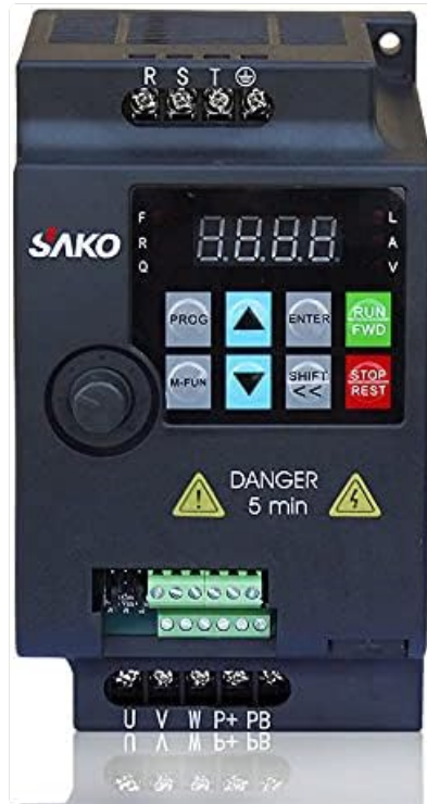
Figure 3.2.1: Front view of the SAKO SKI780 Variable Frequency Drive, showing the digital display, control buttons (PROG, M-FUN, UP, DOWN, SHIFT, ENTER, RUN, STOP/REST), and terminal blocks for power input (RST) and motor output (UVW).
