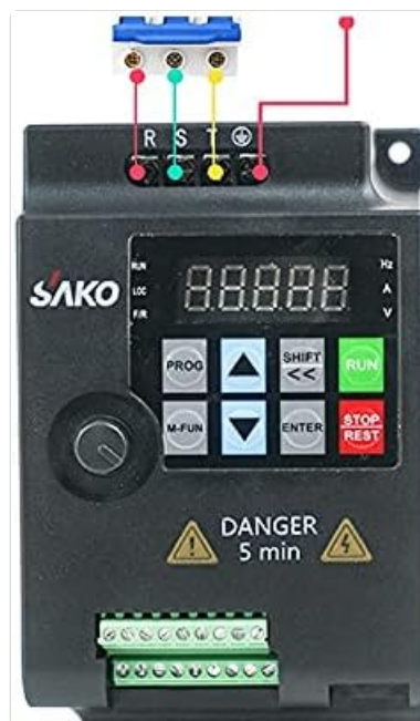
Figure 4.2.1: Wiring diagram for the SAKO SKI780 VFD. R, S, T are for single-phase 220V input. U, V, W are for three-phase 220V motor output. P+ and PB are for braking resistor connections if applicable.
