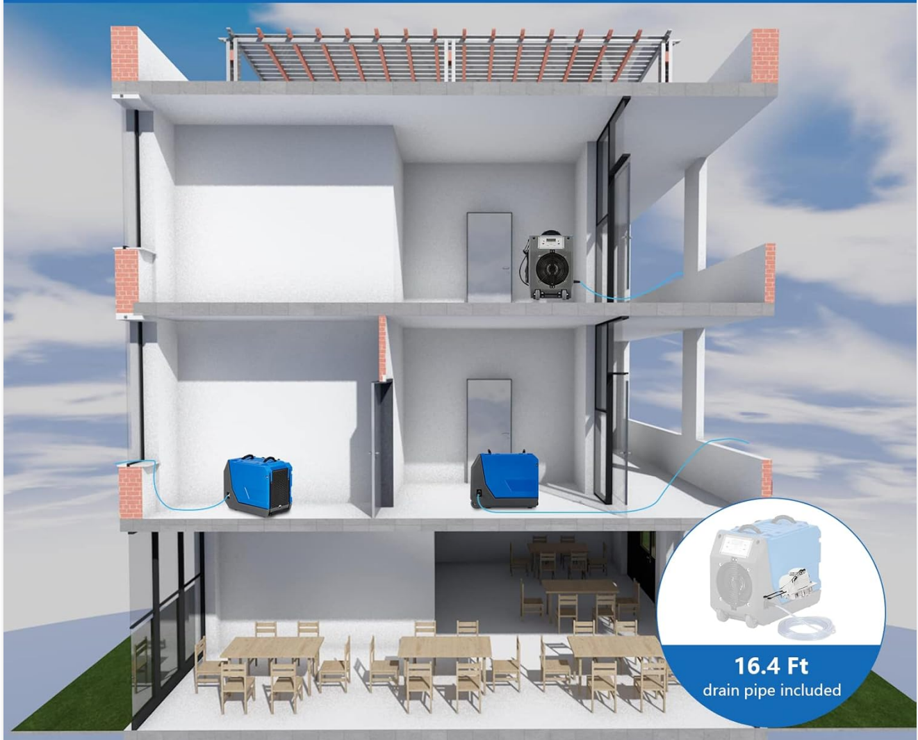
Image 6.1: Illustration of continuous drainage with the built-in pump, allowing water to be discharged to higher levels or distant drains.
