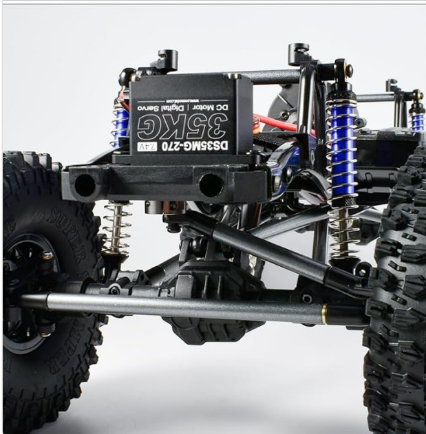
Image 3.2: The 9iMod servo installed in an RC crawler, demonstrating its fit and application.
