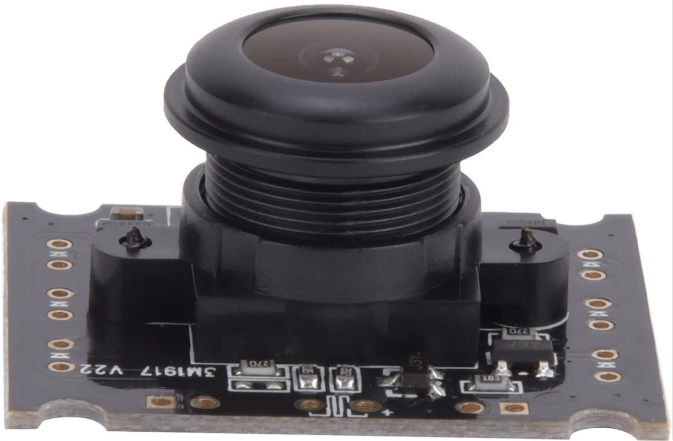
Figure 3.3: Side view illustrating the 110° field of view capability of the USB camera module.
