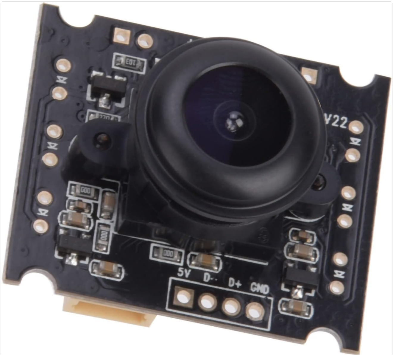
Figure 3.2: Angled perspective of the camera module, showing the lens and board layout.
