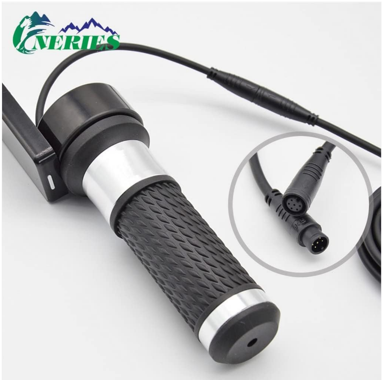
Image: Close-up view of the turn handle and its electrical connector, highlighting the non-slip grip texture.
