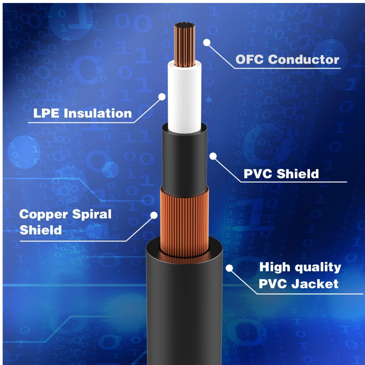
Image 3.1: Internal structure of the CM-04 instrument cable, showing OFC conductor, LPE insulation, PVC shield, copper spiral shield, and high-quality PVC jacket.
