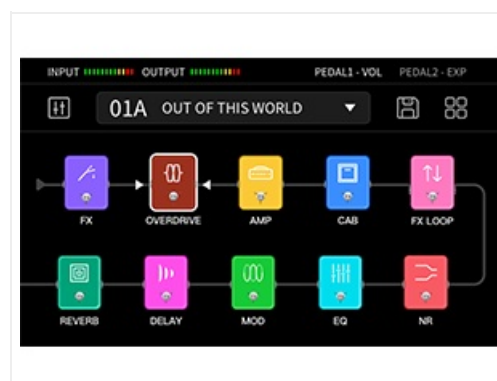
Figure 8: Visual representation of the customizable effects chain on the FX150.
