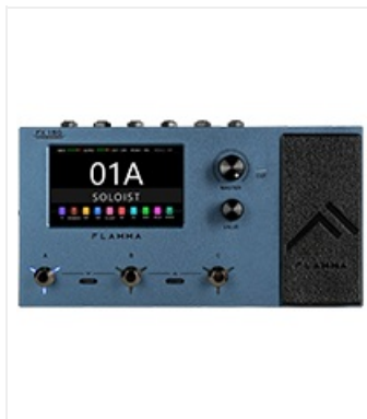
Figure 3: Connect your guitar to the FX150 INPUT. Connect the FX150 OUTPUT to the RETURN of your amplifier's FX Loop or directly to a power amplifier.
