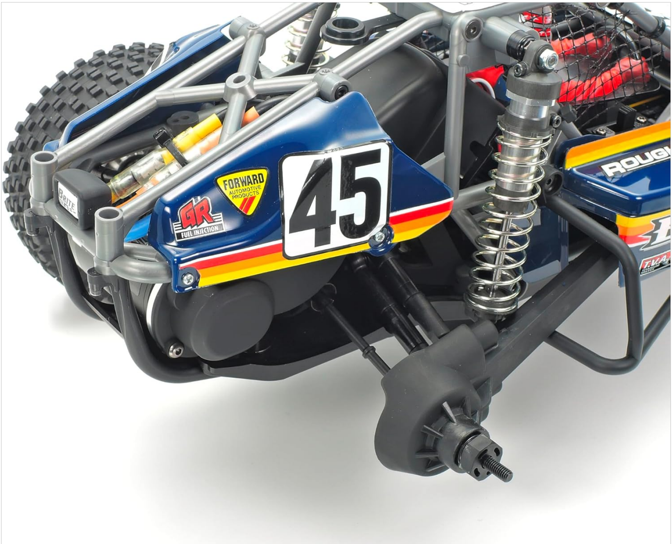
Image 2: Close-up view of the rear suspension and motor area of the TAMIYA BBX BB-01. Note the trailing arm suspension design and the rear-mounted motor for optimal traction.
