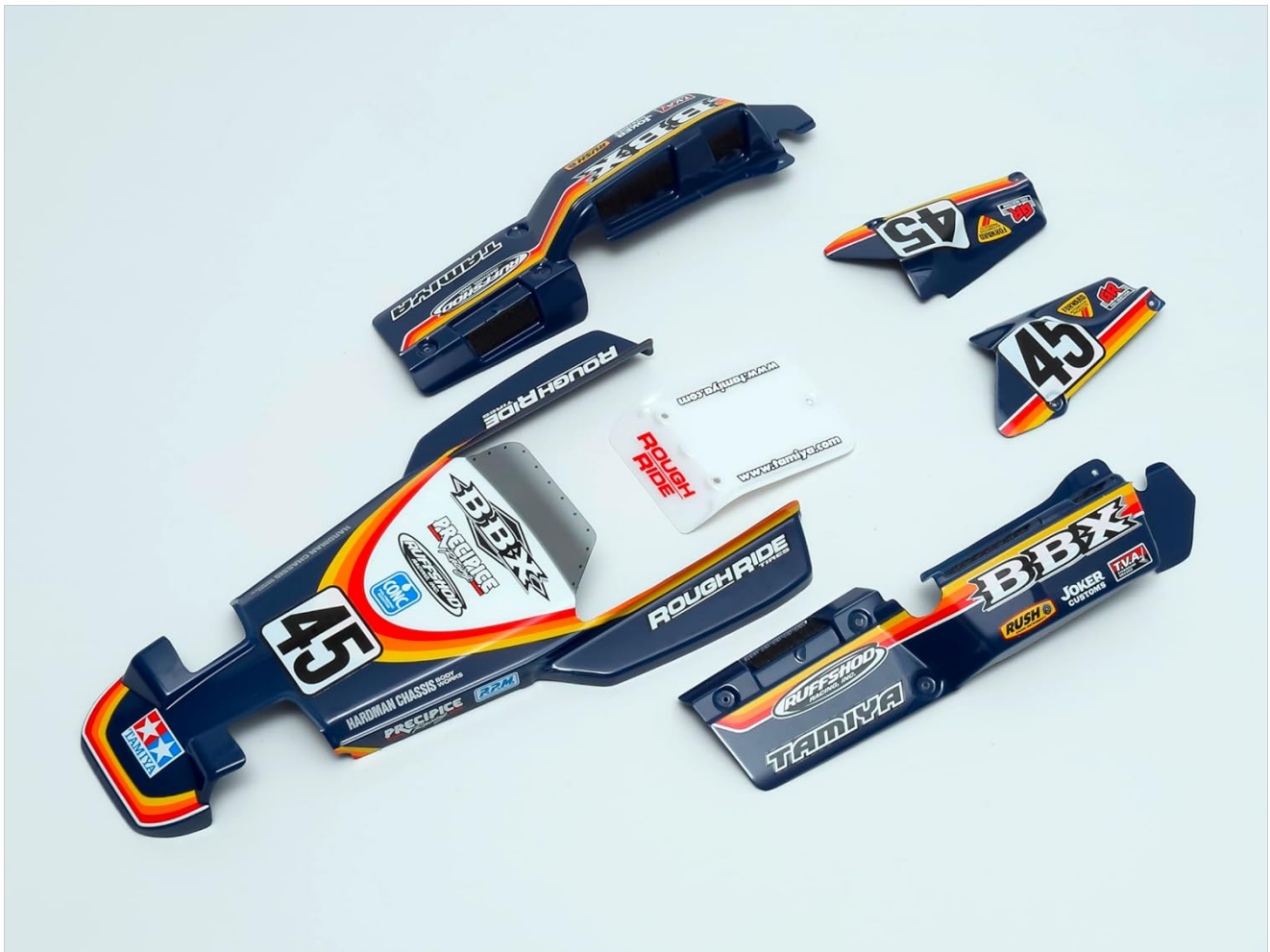
Image 6: The various polycarbonate body sections and decals for the TAMIYA BBX BB-01. These parts are crucial for the model's appearance and should be handled with care during cleaning and reassembly.
