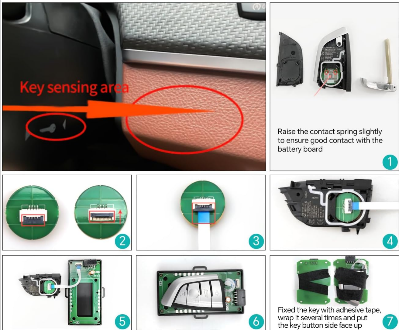
Image 6.1: Detailed visual steps for bypass module installation.
