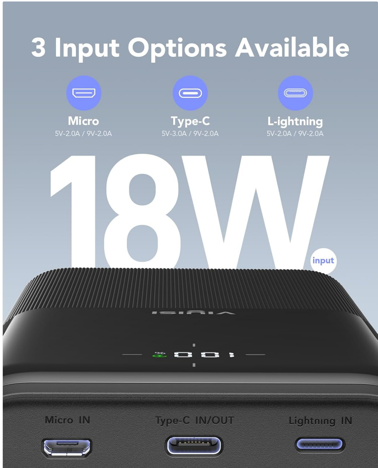
Image 2.2: The three input options (Micro USB, Type-C, Lightning) for recharging the power bank.
