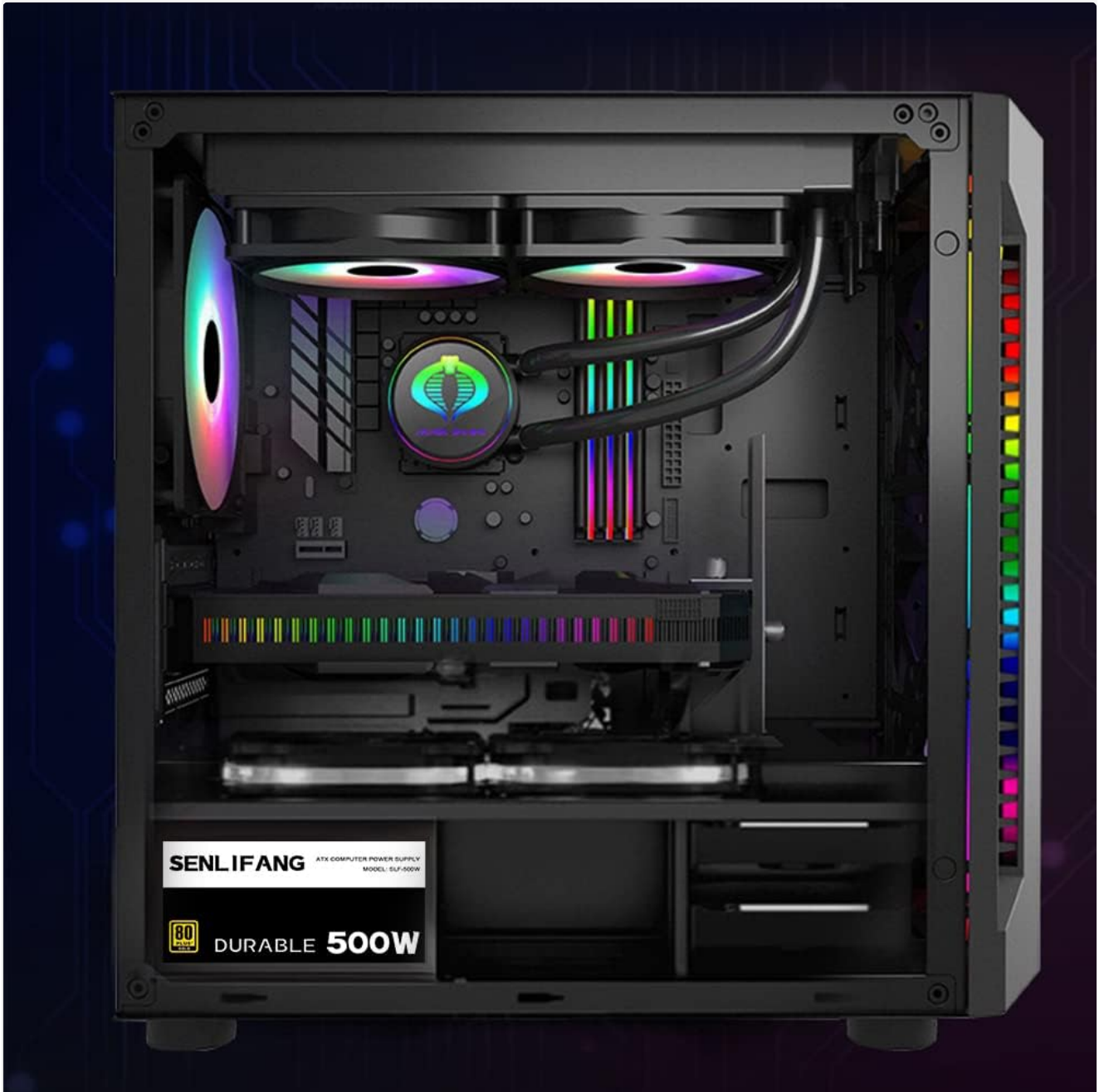
Image 3.1: Example of a power supply installed within a PC case, demonstrating typical placement.
